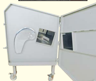
LEFT END DOOR OPEN SHOWING A SICKLE-TYPE SMOOTH BLADE AND THE SURPLUS CATCH TRAY . THE STAINLESS STEEL CATCH TRAY ALLOWS THE FURTHER USE OF THE SLICER'S PRODUCT'S SURPLUS PIECES. USE PIECES FOR STIR FRY, FAJITAS, AND FOR FURTHER PROCESSING LIKE GROUND MEAT. THIS ADVANTAGE QUALIFIES THIS MACHINE TO HAVE A VIRTUALLY ZERO WASTE OPERATION.
