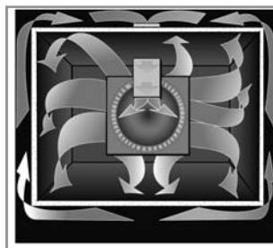
Turbo-Flow provides even heat throughout the oven
